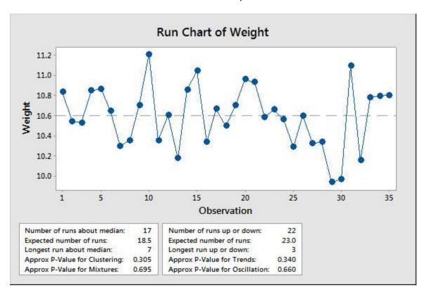
Common cause variation is **the kind of variation that is part of a stable process**. These are variations that are natural to a system and are quantifiable and expected. Common cause variations are those that are predictable, ongoing, and consistent.
